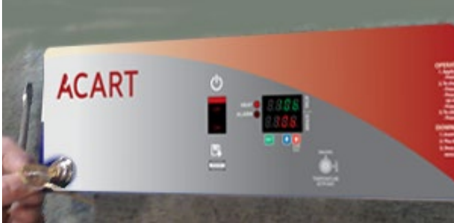
Fig. 37: Overlay - Cam Lock Location - Right Hinged Door
