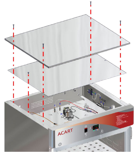
Fig. 29: Remove Top Panels
