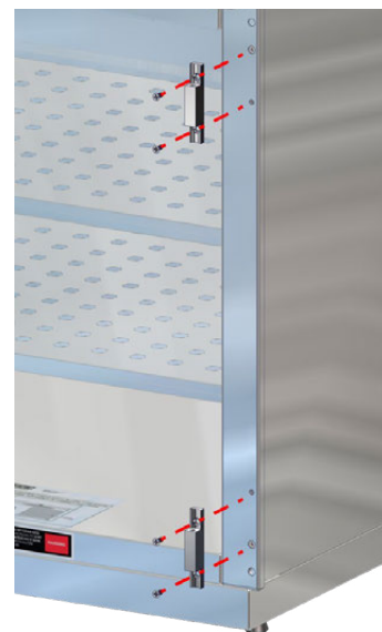
Fig. 46: Detach Glass Door Hinge - Male Half
